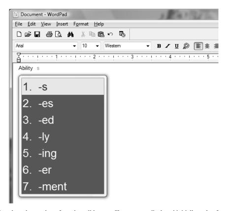
To reduce the number of word candidates, suffixes are not displayed initially, only after you auto-complete a word. After a word is completed, a list of suffixes is displayed (if enabled in WordLists Settings), and can be selected and used the same way as above. Suffixes automatically remove auto-spacing, and built-in suffix rules are used (i.e. remove e if suffix is -ed).
