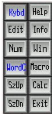
The Control panel allows you to open and close all OnScreen panels. Click on each key to perform the toggle action. Blue (highlighted) letters indicate an open panel, black letters indicate a closed panel. OnScreen also indicates the open panels by latching (or showing as depressed) each panel button. See ControlPanelToggleButton setting in the Initialization file.
